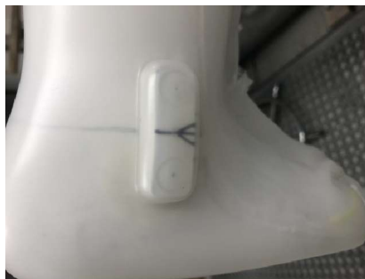
Fig. 4 Note the hole in the dummy through the plastic and trim line
